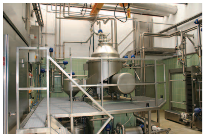
Separator for the production of curd
